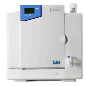
PURELAB Option-R 7/15. This system provides pure water on demand with a range of flowrates suitable for many general molecular genetics applications.
