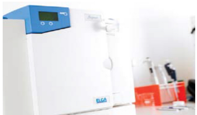
The unit supplies purified water directly to the water disinfecter
